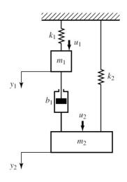
**2** Obtain the Transfer Functions  $X_1(s)/U(s)$  and  $X_2(s)/U(s)$  of the mechanical system shown in the Figure.
